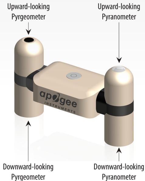
Apogee Instruments' four-component net radiometer consists of an upward-looking and downward-looking pyranometer (to measure shortwave radiation), and an upward-looking and downward-looking pyrgeometer (to measure longwave radiation). Each provide separate measurements of the four components of net radiation.
