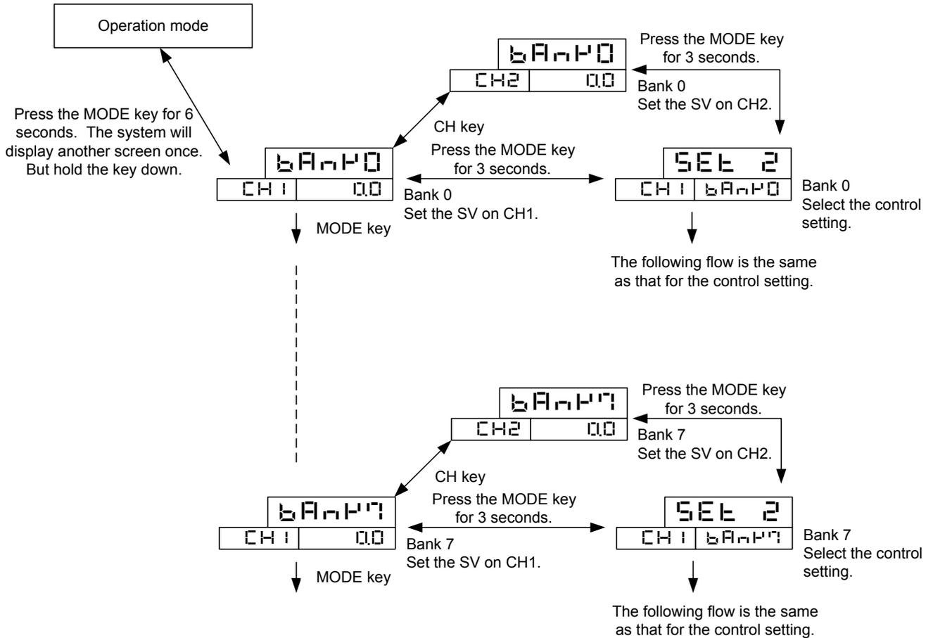
While in the operation mode, press the MODE key for 3 seconds. The system will then switch to the "Select the setting mode" screen. But hold the key down for a total of 6 seconds or more until the system switches to the bank setting mode. The bank setting mode comes in the SV setting mode and the control selection setting mode.
