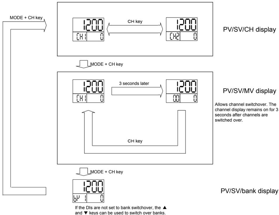
The auxiliary screen in the PV/SV/MV display switches over among CH1MV1, CH1MV2, CH2MV1, and CH2MV2 every time the CH key is pressed.
